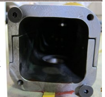
Test pile cross-section Talesnick sensors
