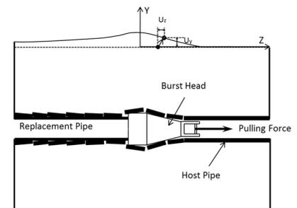
*Schematic of the pipe bursting process and the surface movements*
